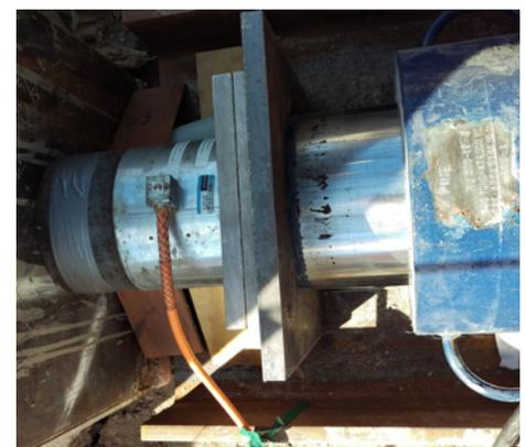
Lateral load test jack and load cell
